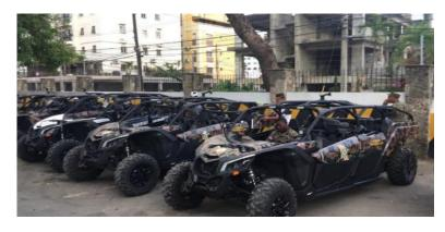
tires and the RPAMS' extended flatbed. The RPAMS run-flat tire has made a name for itself in the UTV industry – in recreational, commercial and military markets. With a reinforced hybrid construction throughout the tire (including the sidewalls), the RPAMS run-flat tire stands up to the harshest environments. Even if it does puncture, it's built to maintain rigidity and run devoid of air for a limited distance at payload.
